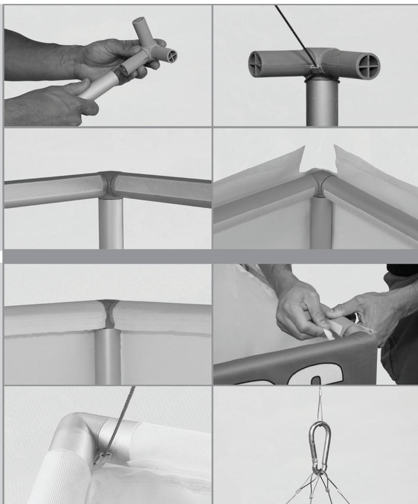
1. Assemble the Aluminum poles (E) and connectors to create the display. The Hanging Square will use the 3D Connector (A) and the Hanging Triangle will use the 60° Connector (B). Slip the bottom of all top connectors through one of the looped ends of the Steel Rope (D).
